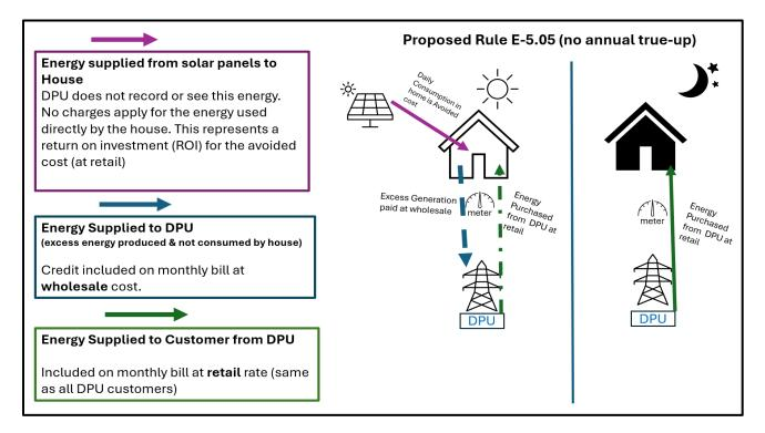
Note: Whether excess generation is supplied to DPU or energy is being purchased from DPU, is determined by the amount of energy produced from a home's solar panels as well as direct consumption by the house.
