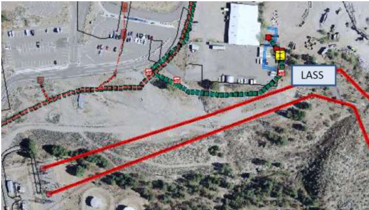
Figure 10. Preferred area for new LASS substation addition
