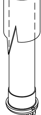
6" PVC RISER PIPE CUT THE REQUIRED LENGTH FROM SEWER SERVICE LINE TO TO GROUND LEVEL
