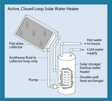
The basic components of a solar water heater system include storage tanks and solar collectors. Active systems have additional circulating pumps and controls, and passive systems do not.
