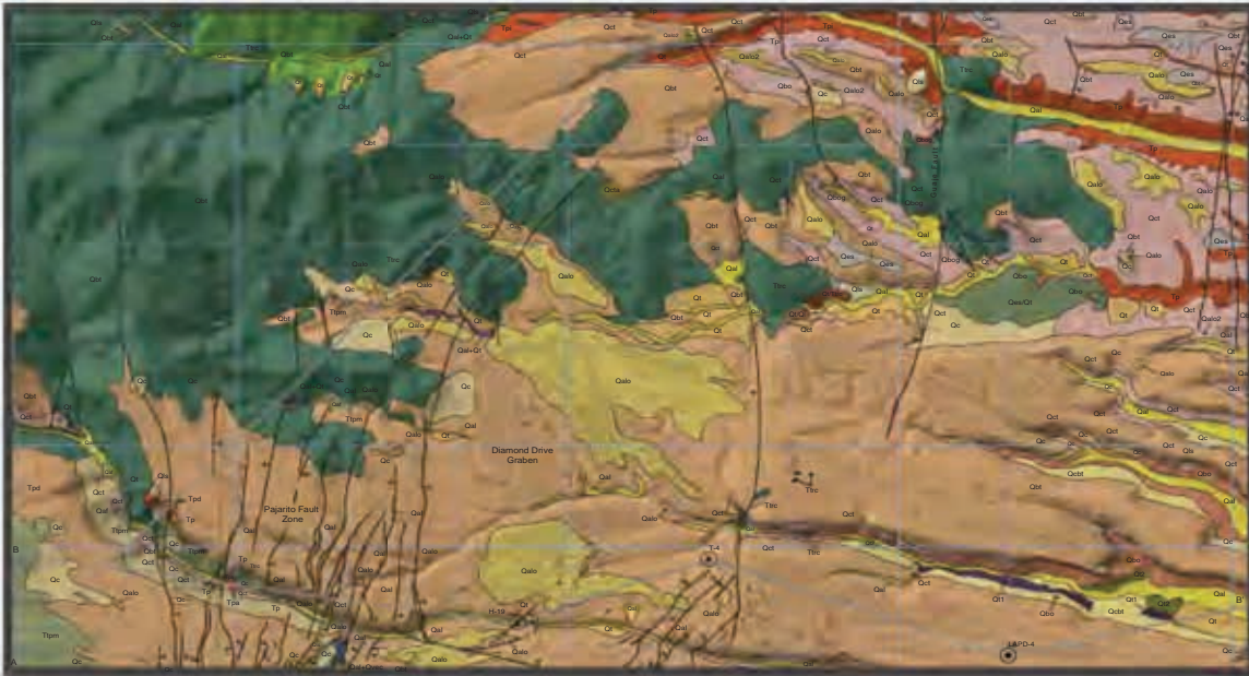
Geologic Map of Los Alamos townsite. Basic interpretation: green designates rhyodacite lava flows; tan designates Bandelier Tuff; yellow, pink, and red designate sedimentary deposits.
