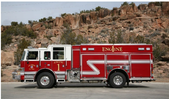
Engine 1 – 1500 gpm Pumper
