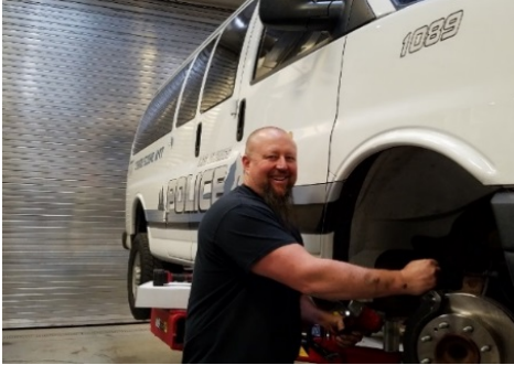
Fleet Technician installing new breaks
