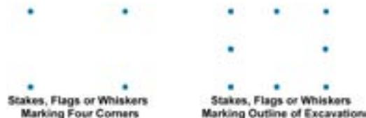
Delineate the proposed area of excavation using stakes, flags, or whiskers instead of spray paint to mark radius or arcs; the four corners of the project; or when outlining the excavation project. Limit the interval spacing to approximately 4 ft to 50 ft. Reduce the separation of excavation marks to a length that can reasonably be seen by the operator's locators when the terrain at an excavation site warrants. Stakes, flags, or whiskers provided to illustrate
